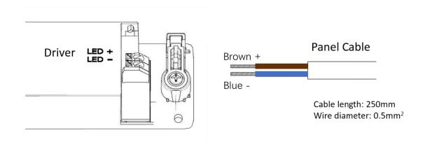
Panel cable must be attached with strain relief protection
